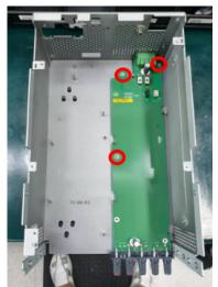
Unsolder the binding post assembly from the IO board. Replace the existing binding post assembly with a new binding post assembly.
