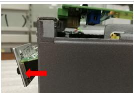
Remove two screws from the insulator using a T10 bit. Remove the insulator.
