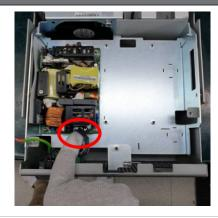
Detach the power PSU connector from the mainboard.
