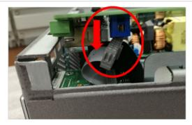
**12** Remove the GPIB module from the chassis.
