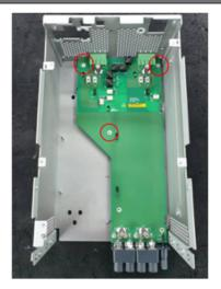
22 Unsolder the binding post assembly from the IO board. Remove the four screws with a T-10 bit. Replace the existing binding post assembly with a new binding post assembly.
