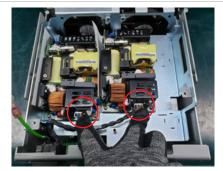
**15** Detach the power PSU connectors from the mainboard.
