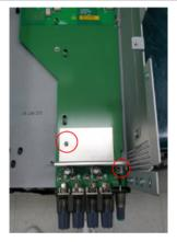
21 Remove three screws from the IO board using a T10 bit. Remove the IO board from the chassis.
