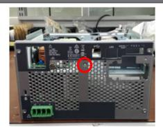
17 Remove two screws from the bracket using a T10 bit. Remove the bracket from the chassis.
