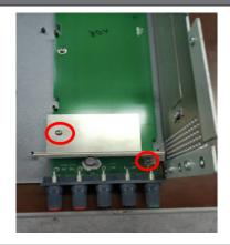
Remove three screws from the IO board using a T10 bit. Remove the IO board from the chassis.
