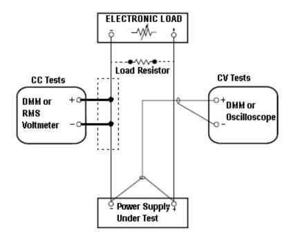
This setup is used for most tests and it requires the DMM, electronic load, and power supply being verified. Some wire is also required for connection between instruments. A LAN or USB cable is needed for readback data. The DMM measures the power supply output, and the electronic load draws current from the power supply. The accuracy of the current monitoring resistor must be 0.01% or better, which should include any self-heating effects.
