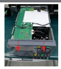
**8** Detach the power PSU connector from the IO board.
