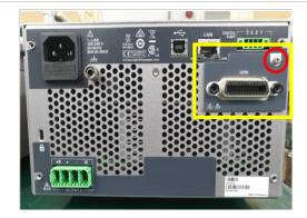
11 Detach the GPIB module connector from the IO board.
