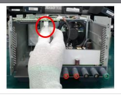
**9** Remove four screws from the IO board using a T10 driver. Remove the IO board from the chassis.
