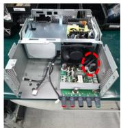
Remove one screw from the rear chassis using a T10 bit.
