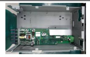
Take caution not to bend any of the connector pins on the IO board.
