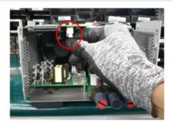
**9** Remove four screws from the IO board using a T10 driver. Remove the IO board from the chassis.
