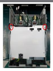
14 Detach the AC inlet connector from the PSU module.
