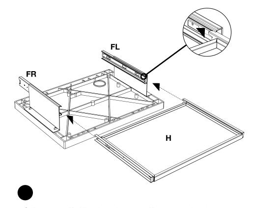
Collect parts: **H**. Align the pullout shelf **H** runner so that the runner snaps into place into the **FL** & **FR** brackets. Pull the shelf out to make sure it is fully seated. Tighten screws **A**. Pullout keyboard shelf assembly is now complete.
