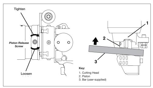
Figure 17, Piston Manual Retract Procedure
