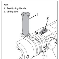
Figure 11, Positioning Handle and Lifting Eye
