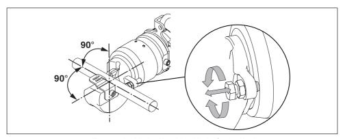
Figure 12, Positioning Material Inside the Cutting Head
