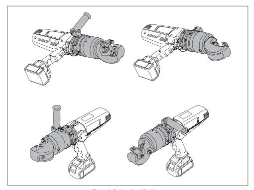
Figure 6, Cutting Head Positions
