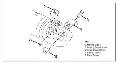
Figure 16, Fixed and Moving Blade Replacement
