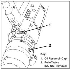
Figure 14, Oil Drain/Fill Cap (cutter shown in inverted position)
