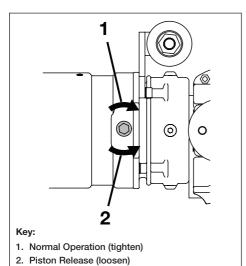
Figure 9, Piston Release Screw
