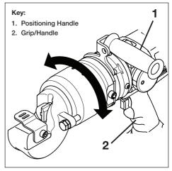
Figure 5, Cutting Head Rotation
