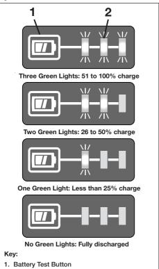
Figure 2, Battery Charge Indicator
