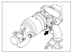
Figure 7, Trigger On-Off Switch
