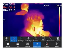
5. Go to **Palettes**, Set **Alarm Temperature (Above)** as required. If the measured value exceeds the set value, the displayed **Max Temp. Value** turns red and flashes, as shown below.
