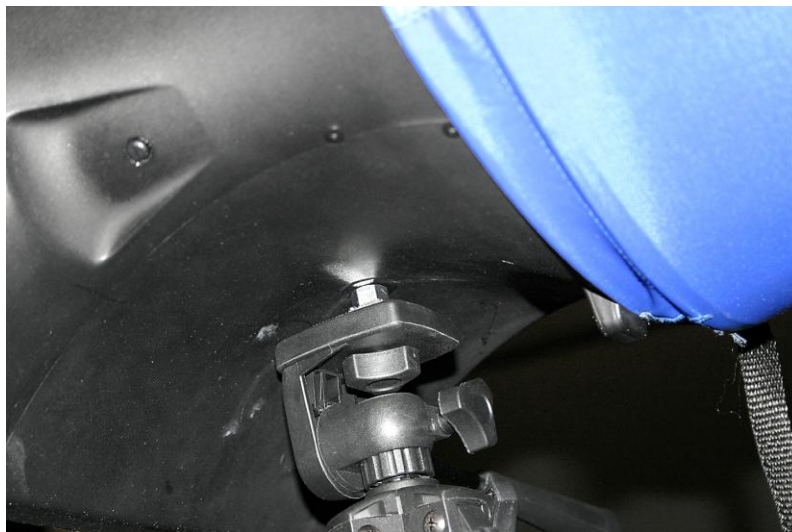
Figure 27: Mount Hood Base to Telescopic Stand
