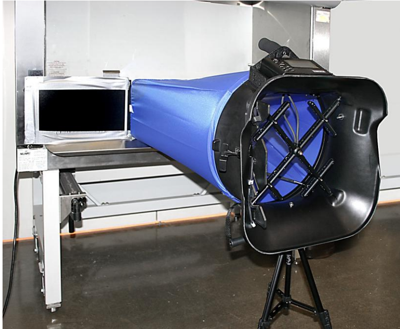
Figure 28: Adjust Height and Position of Telescopic Stand
