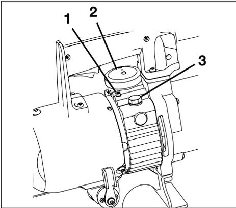
**Figure 13A, Vent Screw (1), Diaphragm Cover (2) and Oil Reservoir Cap (3)**
