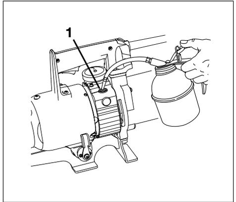
**Figure 13D, Adding Oil to Reservoir Fill Hole (1)**
