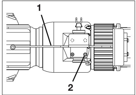
**Figure 14, Standoff Bracket (1) and Directional Control Valve Screws (2)**
