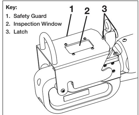
Figure 2, Safety Guard with Inspection Window
