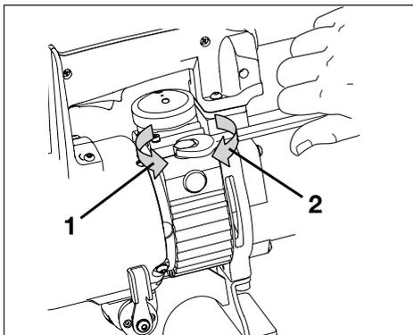
**Figure 13C, Oil Reservoir Cap - Loosen (1) and Tighten (2)**
