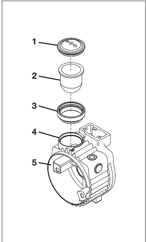
**Figure 13E, Diaphragm Cover (1), Diaphragm (2), Extension (3), Diaphragm Opening (4) and Oil Reservoir (5)**
