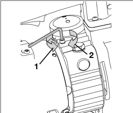
**Figure 13B, Vent Screw - Loosen (1) and Tighten (2)**
