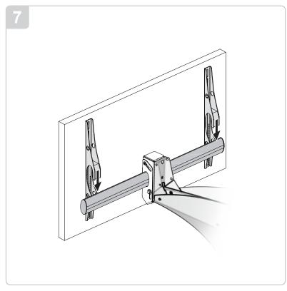
Lower and center the mounting bracket arms with the attached flat panel onto the elliptical mounting bar of the ECM-3000.
