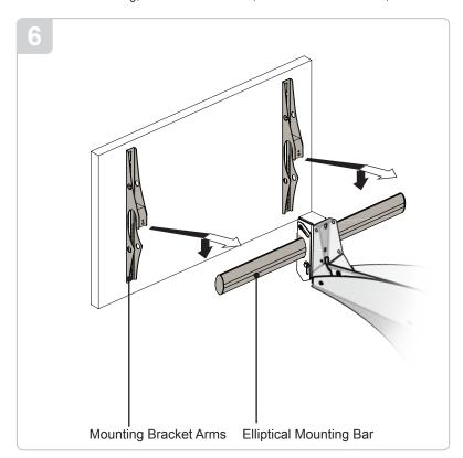
Install the mount according to the instructions provided by Premier Mounts. Ensure all structural reinforcements have been made before attaching the flat panel to the ECM-3000.
