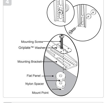
Attach the eliptical tilt mount using four(4) M6 x 6mmscrews
