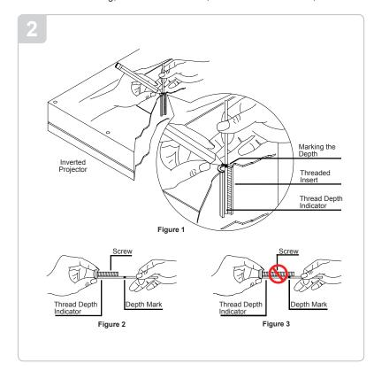
Insert the Thread Depth Indicator into the thread inserts found on the bottom or top of the projector. Use a pencil to mark the depth of the thread insert on the Thread Depth Indicator, as shown. Insert the Thread Depth Indicator into the remaining thread inserts to compare and verify their depth.
