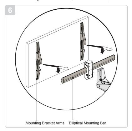
Install the mount according to the instructions provided by Premier Mounts. Ensure all structural reinforcements have been made before attaching the flat panel to the ECM-4000.
