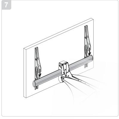
Lower and center the mounting bracket arms with the attached flat panel onto the elliptical mounting bar of the ECM-4000.
