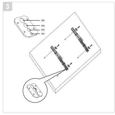
Premier Mounts' Griplate™ Washers are designed to accommodate the various M4, M5, M6 and M8 hole sizes required by flat panels.
