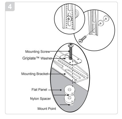
Attach the eliptical tilt mount using four(4) M6 x 6mmscrews
