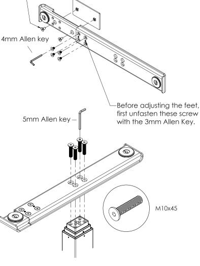
If the table depth is 30" (76cm) or more, expand the top supports on each side.
