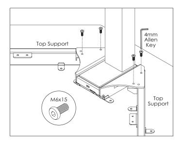
Attach the two-piece side top supports. One piece is attached to the frame; the other piece is separate.
