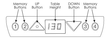
CAUTION: The "zero setting" procedure must be completed before operating the table. See Step 16 on page 8.
