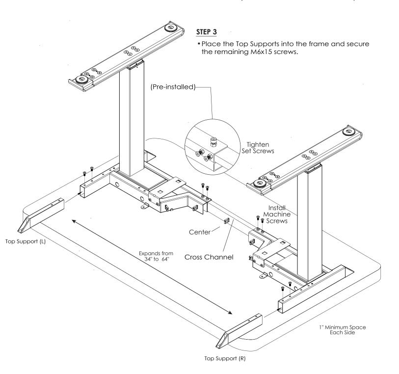
Adjust the position of the frame before screwing it to the work surface.
