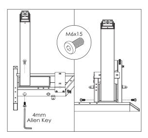
Route the side column motor cables under the notch on the angled portion of each frame.
