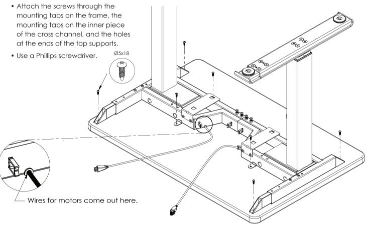
Attach the control unit bracket to the frame and the control unit to the work surface.
