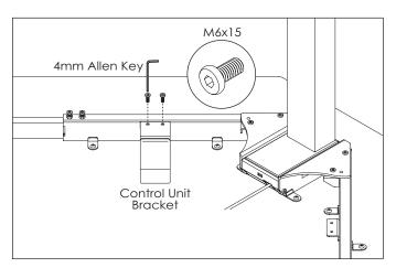
Attach the control unit to the worksurface.
