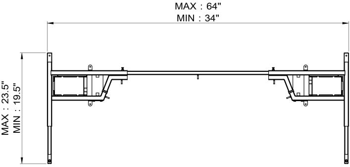
Change the length of the adjustable feet, if necessary.
