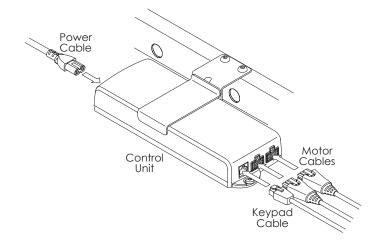
"Zero set" the system before testing operation. (Note that with the table and keypad upside-down, the  $UP \triangle$  and DOWN  $\nabla$  buttons face their opposite directions.)
