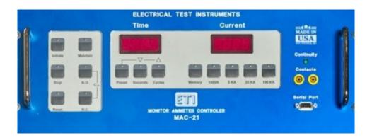
**INITIATE key:** This key is used to turn ON the output of the test set. The LED in the key indicates that the MAC-21 is attempting to turn the output ON. In MOMENTARY mode, the key must be held to keep output current on. In MAINTAIN mode, once current is detected, the output will stay on until the breaker trips, or the STOP or RESET button are pressed.
