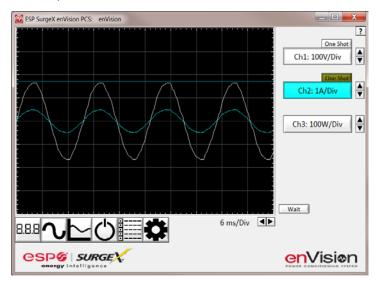
If the Voltage of Current exceeds the trigger level, the scope will hold the display
