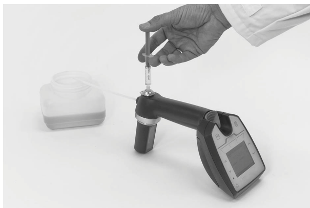
Fig. 12-2: Filling sample using a syringe
