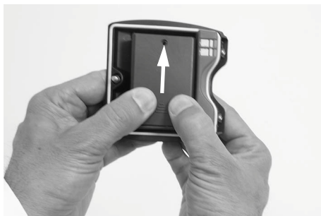
Fig. 15-2: Removing the battery compartment
