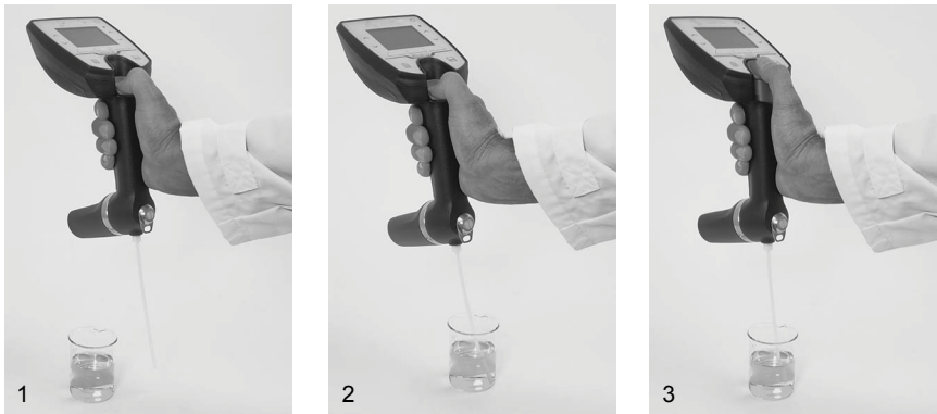
Fig. 12-1: Filling sample using the filling tube
