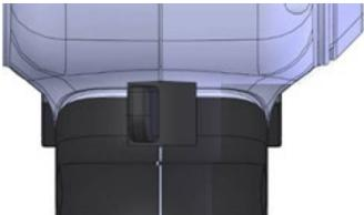
When the switch to the left, the blade goes forward.
