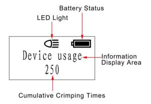
Tool LED illuminator: After pressing the start button, the LED illuminator light will turn on, After the tool is released, the button will automatically turn off after a delay of 20 seconds. Press the start button before installing the battery. When the battery is installed, release the start button and the LED light will turn off. If the light is still on, the battery must be reinstalled immediately as shown in the figure.
