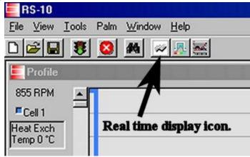
7.1.3. You can now select channels (1 to 10) for viewing. (Note that only the positions that have T type thermocouples connected to Multi Temp should be enabled). If all ten channels are to be displayed, position the mouse cursor over the **Display Meas Temp** box in the **Measurement Profile Window**, click the RH mouse button and select **Set All**. To hide or display each individual channel RH click on the particular measurement profile and select **Add to / Remove** from the profile.
