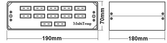
8.3. The Ingress Protection rating for the Multitemp temperature measuring module has been classified as IPX0.
