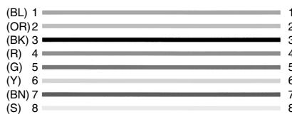
RJ-45 (8-Wire) Straight-Pinning
