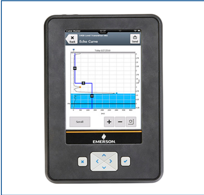
More accurately tune radar measurements with enhanced echo curves.
