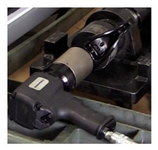
Pull the trigger and record the torque from the readout when the tool stalls.
