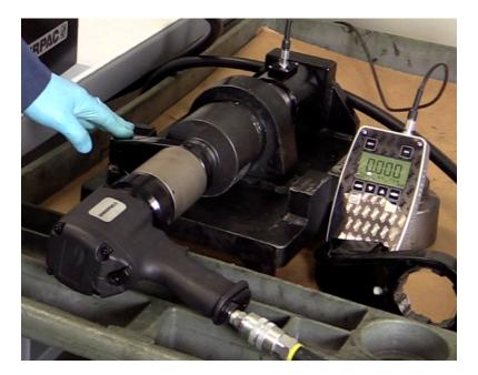
2: Adjust the air pressure to about 10 psi (0.69 bar) below the target pressure with tool free running.
