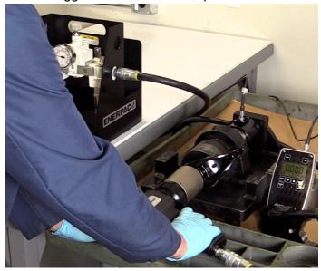
Repeat this process to obtain 3 to 5 data points. The average of these values provides a calibration point. Repeat this process at 10 psi (0.69 bar) increments until the full rated torque of the respective tool is achieved.
