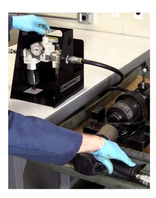
Make sure the reaction arm is secured to the tool and then mount the tool to the calibration stand using the appropriate socket to interface between the wrench square drive and the stand.
