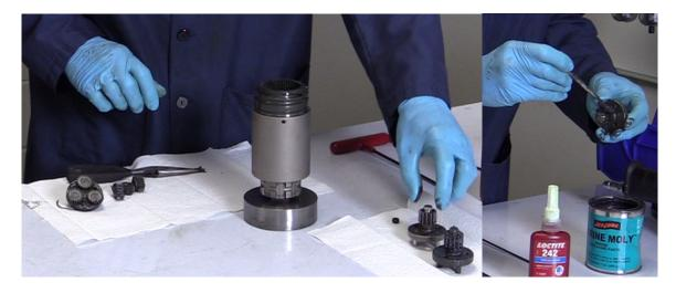
Discard the old second stage gear carrier, then take the new second stage carrier, and apply black Marine Moly™ grease (or similar) generously to the gear teeth, and apply a light coating onto the same face and onto the outside diameter.
