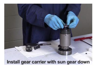
Lower the new second stage gear carrier into the gear housing. Rotate while lowering the carrier to get the sun gear to mesh with the third stage planet gears. Insert the carrier as far as it will go, while ensuring that the sun and planet gears align properly.
