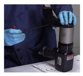
Reattach the reaction arm using a 1/8" Allen wrench to tighten the set screw just far enough that it catches the shoulder of the spline. Do not overtighten.
