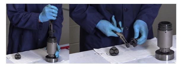
Repeat the previous step to remove the second stage carrier. Note that the second stage planet gears need to be removed, as they will be reused. The second stage gear carrier is the part to be replaced.
