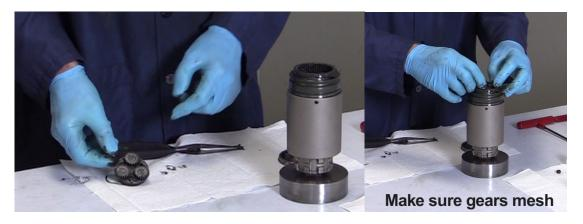
Install the 1<sup>st</sup> stage carrier in a similar manner. When finished, the planet gear surfaces should be flush or below the top rim of the gear housing.
