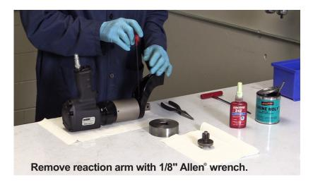
Position the wrench with the top facing down. Remove the reaction arm using a 1/8" Allen® wrench to unscrew the set screw.
