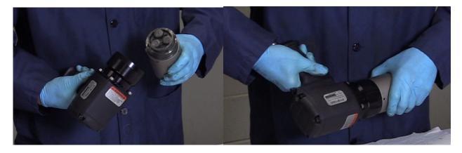
Place the motor adaptor housing over the gear housing and rotate to aide axial assembly. This should be done with the tool in a horizontal working position to avoid the gear stages from coming out of the gearbox, or the washer from coming out of the motor adaptor. First, align the teeth of the sun gear to the first stage planet gears, then seat the O-ring into the adaptor. Observe the ball groove through the set screw hole to verify that the parts are completely joined together.
