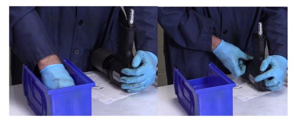
Insert the 35 balls through the set screw hole; occasionally rotate the gear box to get the balls to drop, or hand-press the balls if necessary.
