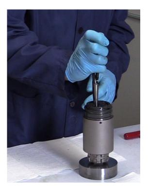
With the gearbox standing on the output end (A drive socket can be used as a fixture to support the gearbox: use a 3/4" socket for the TW1000-75; use a 1" socket for the TW1000, TW2000 and TW3000; use a 1.5" socket for the TW6000). Use a needle nose pliers to lock on to two of the three holes spaced evenly between the planets in the first stage carrier. Pull the carrier assembly upward out of the gear housing.
