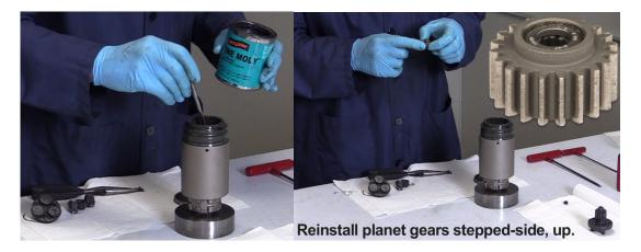
Add grease generously to the three pins on the upper side of the carrier and coat the remaining surface. Slide the planet gears onto the pins of the second stage gear carrier. **Important Note:** The gears are not symmetric. There is a step down diameter on one end. The step down diameter should be away from the carrier (facing up) when sliding on to the pins.
