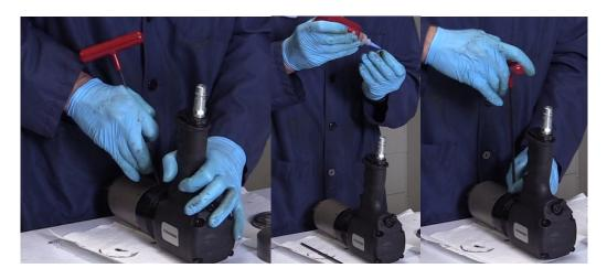
After installing all 35 balls, push the balls to either side of the hole using an Allen Wrench so that there is an open space under the set screw. Apply a drop of Loctite<sup>®</sup> 242 to the set screw, and fasten down the set screw in until it contacts the ball race. Then back out the set screw a quarter turn.
