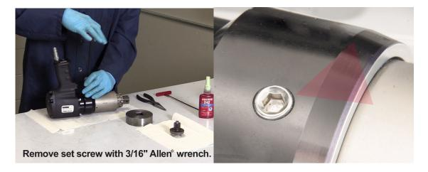
Remove the gear box by unscrewing the set screw on the bottom of the adapter housing with a 3/16" Allen® wrench.
