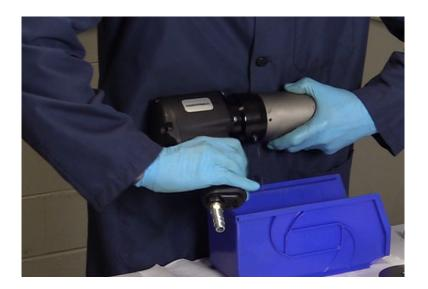
Allow the 35 rotary joint balls to fall out of the adapter through the set screw hole by holding the tool in a horizontal working position and rotating and oscillating to get the balls to drop out. Applying axial forces while rotating can aide this process.
