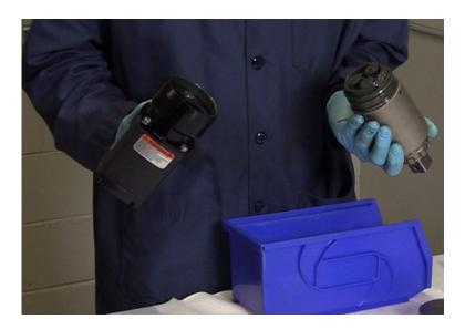
With the balls removed, the gear box will separate from the adaptor. Be sure to hold the gearbox with the output end angling down to prevent the gear stages from falling out.
