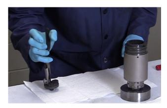
Carefully set the first stage carrier onto a clean towel. Note that the planet gears are not retained axially, and can slide off.
