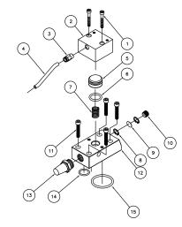
ITEM DESCRIPTION QTY BOLT 2 1 AIR PISTON COVER 2 1 AIR COUPLER 2 3 4 AIR HOSE 1 AIR PISTON 5 1 O-RING 6 1 SPRING 7 1 8 C-RING 2 9 FILTER 1 10 BOLT 1 BOLT 11 4 OIL OUTLET VALVE SEAT 12 1 AIR FILTER 13 1 14 **O-RING** 1 15 **O-RING** 1
