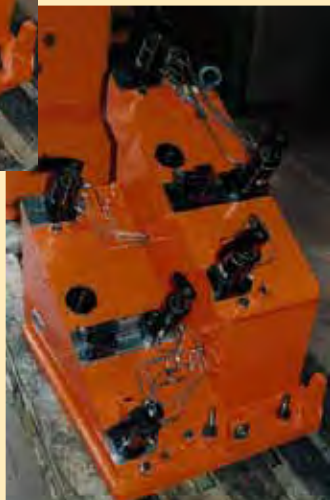
■ MPTL-100 and MPTR-100 Collet-Lok® Swing Clamps are used to securely clamp these exhaust manifolds.
