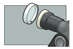
Screw in the Foot Extension fully until the screw-thread is no longer taking load and the foot feels slightly loose:
