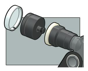
Fit the plastic cap onto the Foot Extension:
