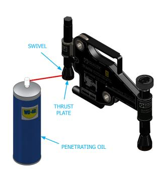
Ensure the thrust plates rotate freely before using the tool to align a flange joint.
