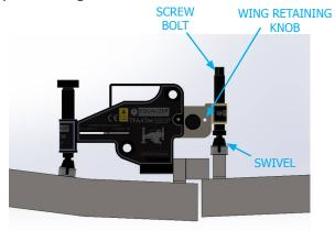
The torque wrench should be set at 19 N·m (14 ft·lb) then attached to the screw bolt.
