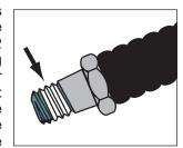
Figure 2: Sealing Tape
