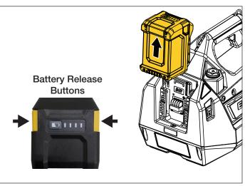
Figure 8: Battery - Remove
