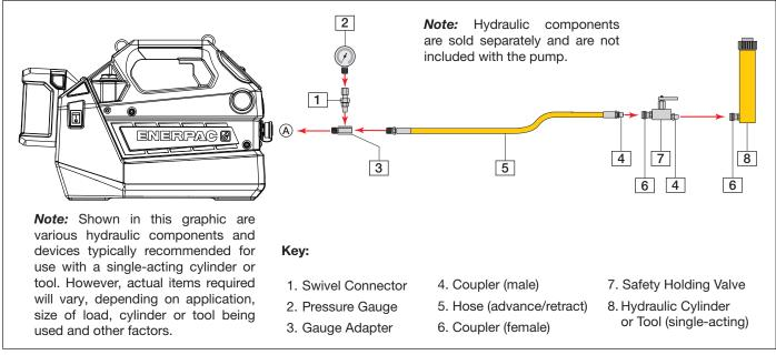
Figure 4: Single-Acting Hydraulic Circuit and Components (typical)
