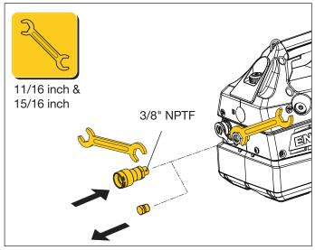
Figure 3: Hydraulic Connection to Pump
