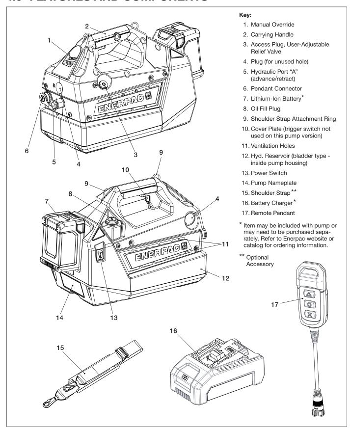
Figure 1: Features & Components, Models XC2302S and XC2304S
