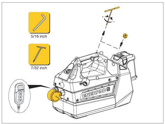
Figure 15: Relief Valve Pressure Adjustment
