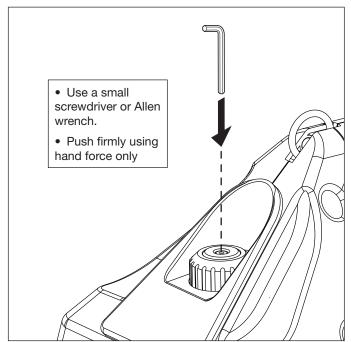
Figure 11: Manual Override Button (pressure relief)
