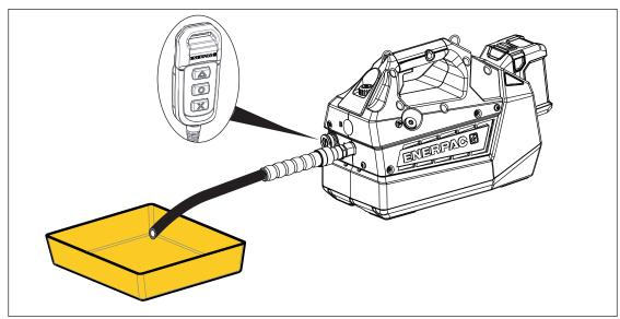
Figure 14: Draining the Hydraulic Reservoir
