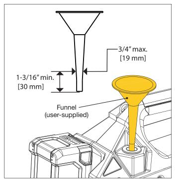
Figure 13: Adding Oil Using Funnel
