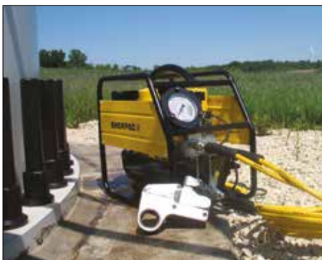
◀ The TQ-700E and the W-Series wrenches are a productive combination in wind applications.
