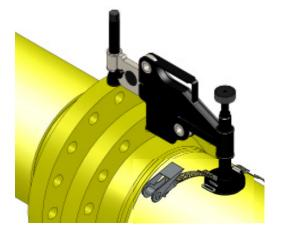
Feed the open end of the strap through the ratchet mechanism as shown. Tighten the strap using the ratchet mechanism.
