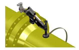
Now place the hook of the ratchet mechanism through the base on the opposite side as shown.
