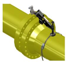
Connect the hydraulic pump to the hydraulic hose, and the hose to the hydraulic adjusting cylinder.
