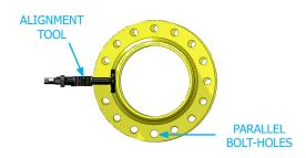
**2.** Insert the bolt into the aligned bolt-hole and release the alignment tool. The load will transfer onto the bolt.
