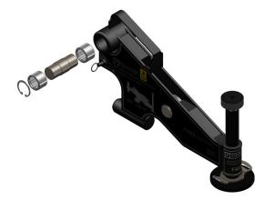
Remove the spiral retaining clips from the lower shaft and slide the shaft out from the main body.
