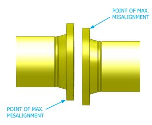
Guide the lift hook into the bolt-hole at the maximum point of misalignment.
