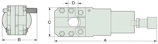
\* HCCS models feature one 3/8" NPT female coupler, HCCD model features two 3/8" NPT female couplers
