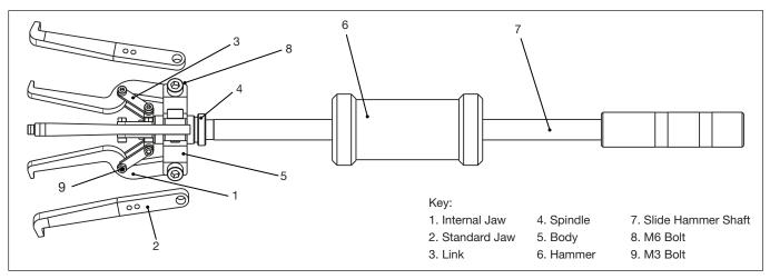
Figure 1: Features and Major Components of the IPM3
