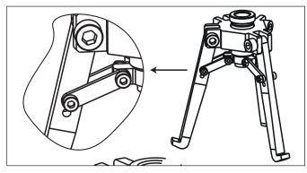
Figure 2: Installation Detail for the Standard Jaw, Internal Configuration
