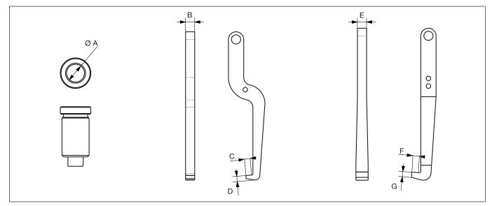
Figure 9: Major Dimensions - Spindle and Jaws
