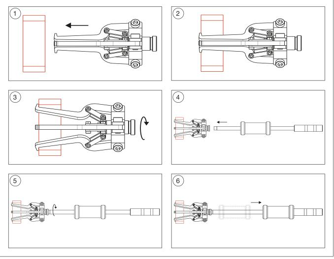
Figure 5: Puller Operation Steps. Extracting an Internal Part.
