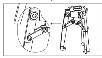
Figure 3: Installation Detail for the Standard Jaw, External Configuration
