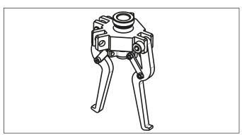
Figure 4: Internal Jaw with Two Jaw Configuration
