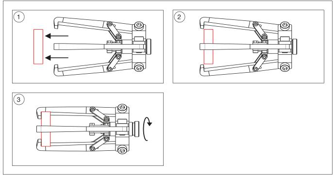
Figure 6: Puller Operation Steps. Extracting an External Part.
