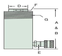
\* R50 Base Mounting hole 7/32 through x 23/64 "C" bore (1/4" depth).
