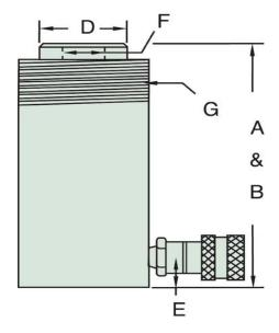
\* R50 Base Mounting hole 5.56 mm through x 9.13 mm "C" bore (10.64 mm depth).
