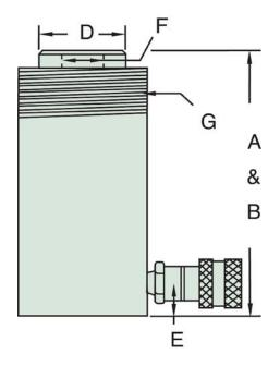
\* R50 Base Mounting hole 7/32 through x 23/64 "C" bore (1/4" depth).
