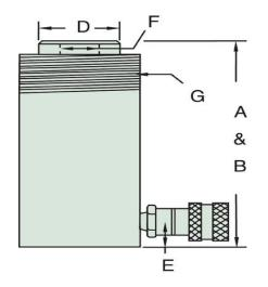
\* R50 Base Mounting hole 7/32 through x 23/64 "C" bore (1/4" depth).
