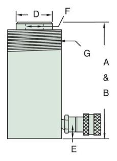
\* R50 Base Mounting hole 7/32 through x 23/64 "C" bore (1/4" depth).
