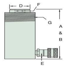
\* R50 Base Mounting hole 5.56 mm through x 9.13 mm "C" bore (10.64 mm depth).
