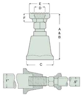
▲ The spreader jack can easily be extended by fitting a .5 in. diameter pipe in the cap well and a 1 in. diameter pipe in the housing well.
