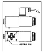
The valves can be mounted to any standard valve manifold with a D03 or CETOP03 mounting pattern. D03 requires the use of #10-24 bolts. CETOP03 requires the use of M5 x 0,8 mounting bolts. lf additional accessories valves are mounted underneath the directional valve, longer bolts will be required. Contact Enerpac for bolt specifications depending on the type and number of accessories installed. Installation torque should be 40-50 in-lbs.
