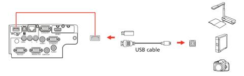
If you connect a digital camera, USB flash drive, or USB storage device, you can use the projector's PC Free feature. See the online *User's Guide* for details.
