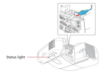
Press the opening power button on the projector or remote control. The projector beeps, and the Status light flashes blue and then stays on.
