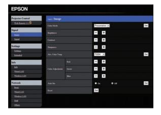
From the Projector Control menu, select **Web Remote**. Use the on-screen buttons to operate the projector, as you would using the remote control.
