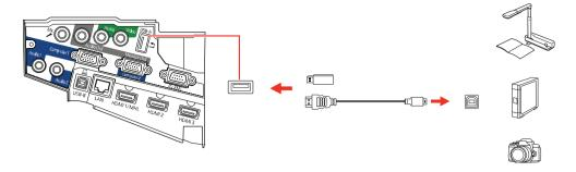
If you connect a digital camera, USB flash drive, or USB storage device, you can use the projector's PC Free feature. You can also connect other Epson document cameras to the projector. See the online *User's Guide* for details.
