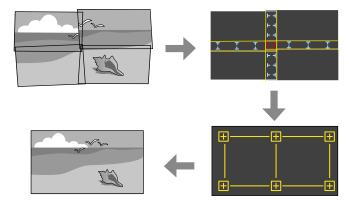
• **Geometry Correction Assist - Stacking Function** wizard allows you to easily and quickly create bright image by overlapping the images of multiple projectors. By adjusting the approximate size and position of your projected image, the projectors automatically overlap these images as one image.
