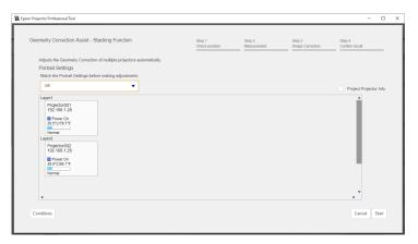
7. Follow the on-screen instructions to adjust the image positions using the **Lens Control** options, so that projected images from multiple projectors roughly overlaps.
