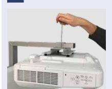
Attach the projector to the arm and tighten the screws.
