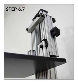
**Step 6:** Position the Monitor Shelf below the lifting assemble and align the holes in the Monitor Shelf with the threaded holes in the Monitor Lifting Assembly.
