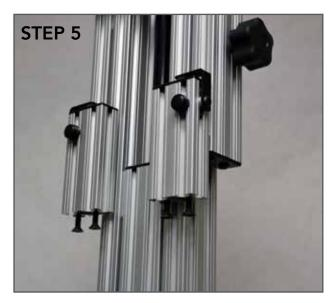
**Step 5:** Loosen both brakes and bring the unit to its full height. Re-tighten the brakes to hold position. Remove the (4) 1/4-20 x 1.0 flat head bolts from the bottom of the Monitor Lifting Assembly.
