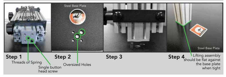
**Step 1:** Lay the lifting assembly on a solid surface with the back side up as shown. Notice the single Button Head Bolt in the assembly union plate. DO NOT LOOSEN THE SINGLE BUTTON HEAD BOLT THAT IS NOTATED.
