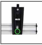
To move the mount horizontally closer or farther apart, simply loosen the bolt attached to the horizontal monitor rail (D) by a single turn with an 5/32 allen wrench. Once you have reached the desired position tighten the bolt.
