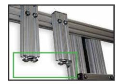
**Step 10:** Remove the (4) 1/4-20 x 1.0 hex head bolts and (4) washers from the bottom of the Monitor Lifting Assembly.
