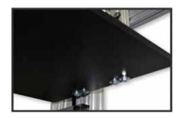
**Step 12:** Thread the (4) hex head bolts into the threaded holes in the Lifting Assembly to secure the laptop shelf to the unit. Tighten securely with a 7/16 wrench.
