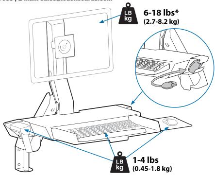
\*The Combo Arm can be modified to mount displays up to 25 lbs (11.3 kg), however display lift and tilt motion will not be possible if this option is chosen. Refer to special instructions on page 7.
