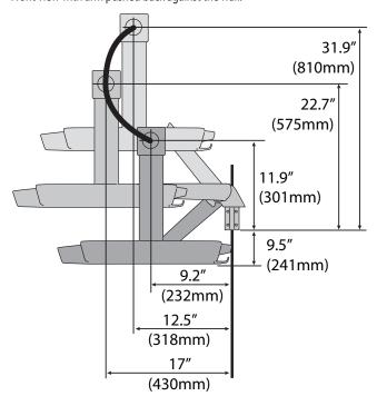
Top view showing range of motion when pulled out from the wall.
