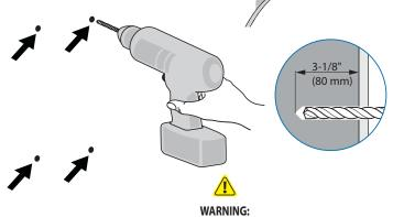
Mounting holes must be at least 3-1/8" (80mm) deep and must be located within solid concrete, not mortar or covering material. If you drill into an area of concrete that is not solid, reposition mounting holes until both anchors can be fully inserted into solid concrete!
