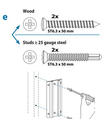
NOTE: Fasteners may unwind due to vibration caused by movement of mounting solution over time. Inspect mounting solution for loose fasteners on a routine basis. If desired, apply a light duty thread locking adhesive to fasteners before installation to prevent back-out.
