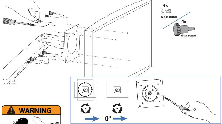
WARNING! Stored Energy Hazard: The arm mechanism is under tension and will move up rapidly, on its own, as soon as attached equipment is removed. For this reason, DO NOT remove equipment unless the arm has been moved to the highest position! Failure to follow this instruction may result in serious personal injury and/or equipment damage!
