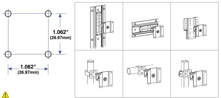
NOTE: Fasteners may unwind due to vibration caused by movement of mounting solution over time. Inspect mounting solution for loose fasteners on a routine basis. If desired, apply a light duty thread locking adhesive to fasteners before installation to prevent back-out.
