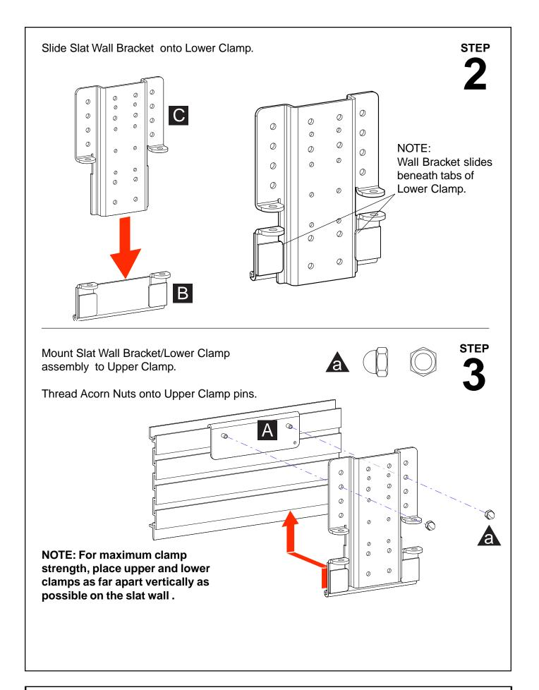
Using a 3/8" wrench, tighten Acorn Nuts.
