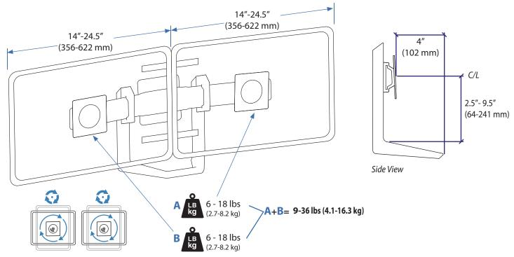
This product adds an additional 6 lbs (2.7 kg) to your mounting solution. Your mounting solution's monitor weight capacity must be reduced by 6 lbs (2.7 kg) when using standard monitors less than or equal to 2.5" (64 mm) thick. Additional reduction will be required if monitors are greater than 2.5" (64 mm) thick.
