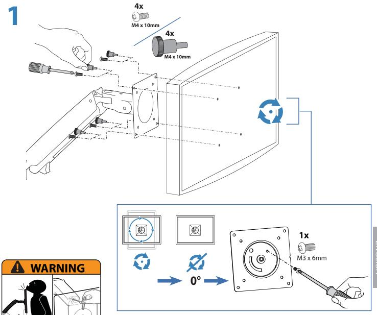
WARNING! Stored Energy Hazard: The arm mechanism is under tension and will move up rapidly, on its own, as soon as attached equipment is removed. For this reason, DO NOT remove equipment unless the arm has been moved to the highest position! Failure to follow this instruction may result in serious personal injury and/or equipment damage!
